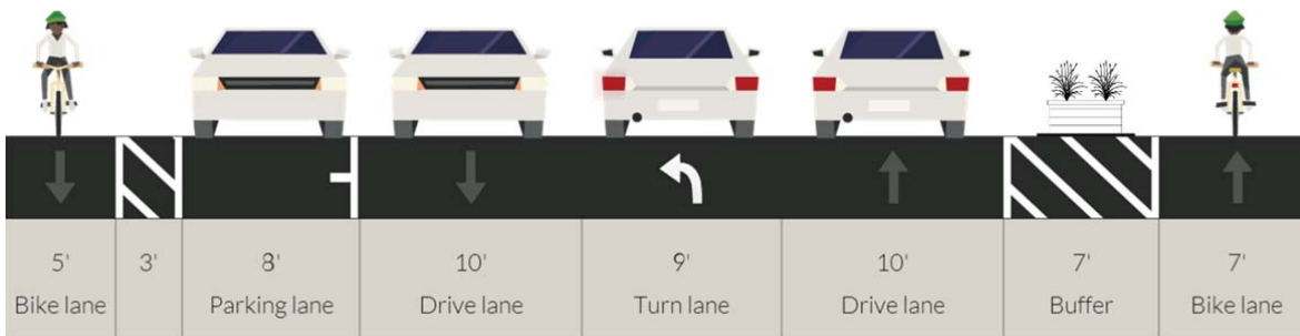
Figure 3-27. Sample Cross section of NE Multnomah Protected Bike Lanes
