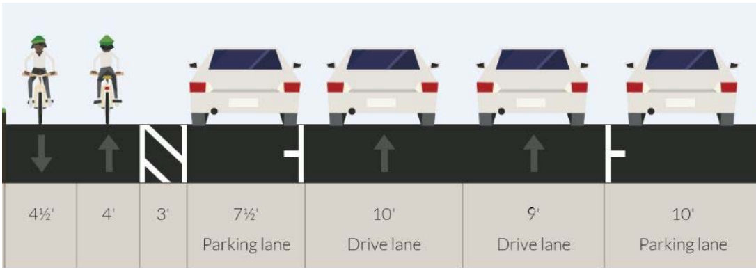
Figure 3-18. Sample Cross section of Dearborn Street Protected Bike Lanes
