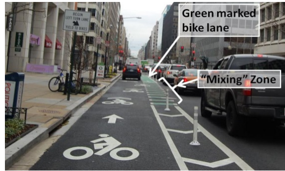
Turning Zone with Post Restricted Entry and Through Bike Lane (TBL) Photo from survey (shown): L Street Video Location(s): L Street/ 15th Street, L Street/ Connecticut
