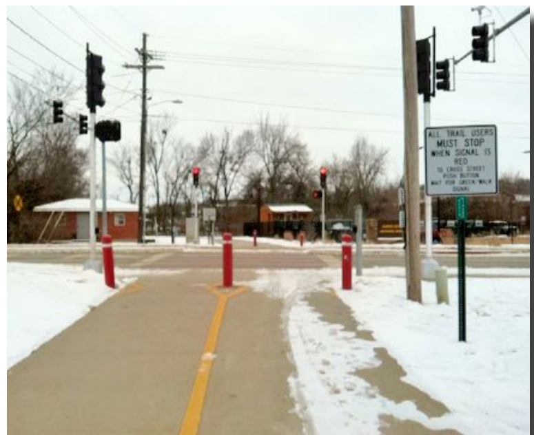
Above: Intersection of street and trail in Fayetteville, AR. Cyclists and walkers can push a button to initiate a stoplight for street traffic in order to cross. Image credit: Rebecca Zimmermann
