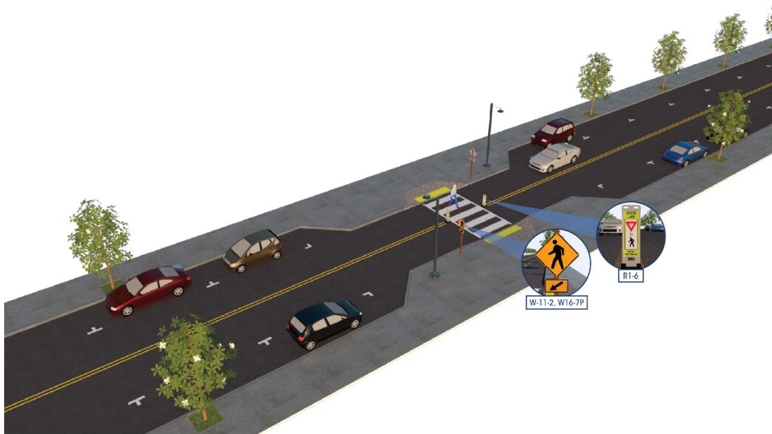
Figure 14. Curb extensions to a mid-block crosswalk.
