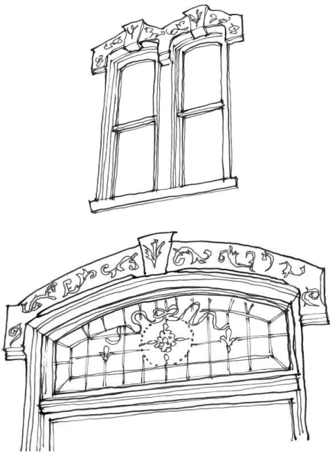
Figure 17. Historic decorative stained glass windows and window hoods should be preserved and maintained.
